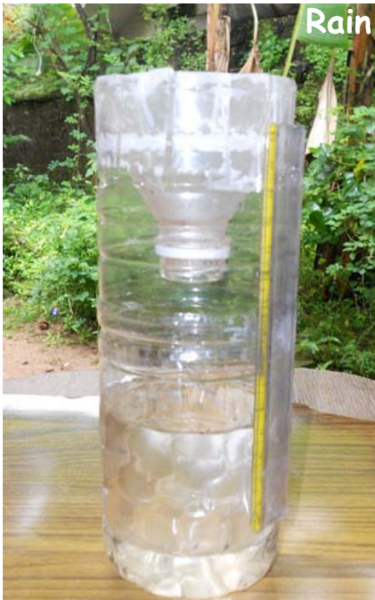
Homemade rain gauge, photo by Fotokannan
